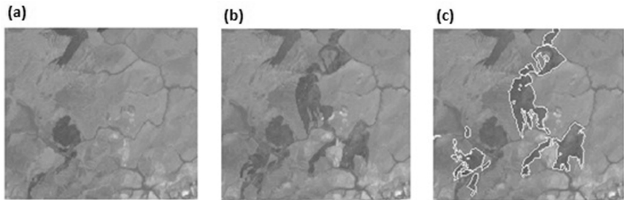
Figure 1. Delimitation of burned area by using a subset of Landsat image 005/056: (a) shows the first acquisition Landsat image of the pair (2003/01/06), (b) shows the second acquisition Landsat image of the pair (2003/01/22) where the burned area can be visually identified, (c) shows the burned area identified between acquisitions
